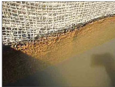
Figure 3. Matting used for floc collection
