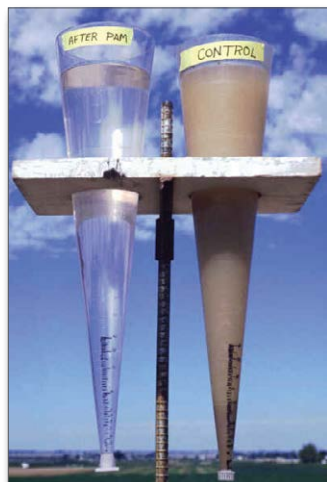
Figure 24. Comparison of water from furrows with and without PAM
