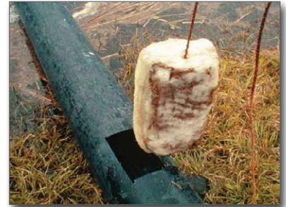
Figure 19. Polymer blocks inserted into pipes
